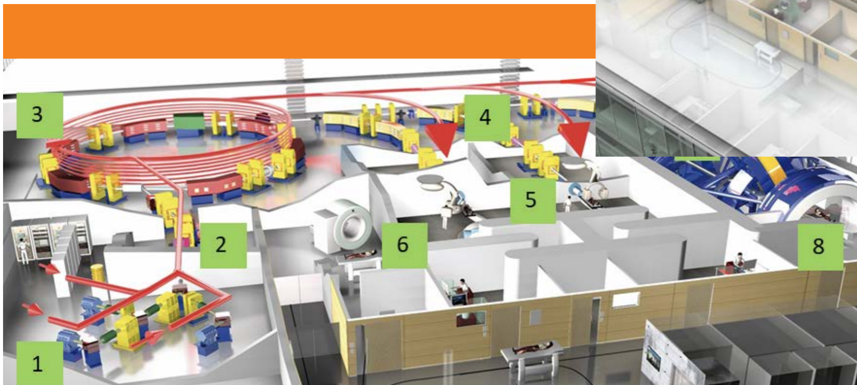
Figure 4: The (1) ion sources: beams of positively charged ions are generated. Hydrogen gas is used to extract protons and carbon dioxide is used to extract carbon ions. Helium gas is used to extract helium ions. (2) Ions are accelerated in high-frequency structures to a tenth of the speed of light. (3) Synchrotron: Six 60° magnets keep the ion beams on a circular path. During around one million orbits, the speed of the ions is increased to up to 75% of the speed of light. (4) On the way to the treatment room: The therapy beam is guided and bundled by magnets in vacuum tubes. (5) The patient is placed on a radiation table that is precisely adjusted by a computer-controlled robot. (6) Position control: With a digital X-ray system and/ OR CT, images are generated before the irradiation. A computer program compares this with the treatment planning for the exact adjustment of the patient. (7) The gantry: With the rotatable radiation source, the therapy beam can be directed at the patient at the optimal angle. The gantry weighs 670 t, 600 t of which can be rotated with sub-millimeter precision. (8) Treatment in the gantry: Two rotating digital X-ray systems enable the position to be checked before the irradiation. (9) Beam guidance to the experimental area, e.g. for irradiation of tissue phantoms, cell cultures, mice and various other measurements.
