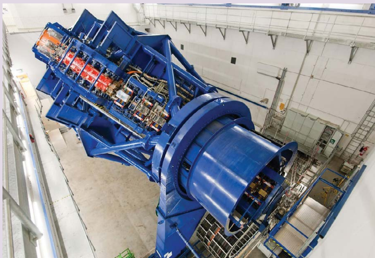
Heidelberg Ion Beam Therapy Centre gantry.
