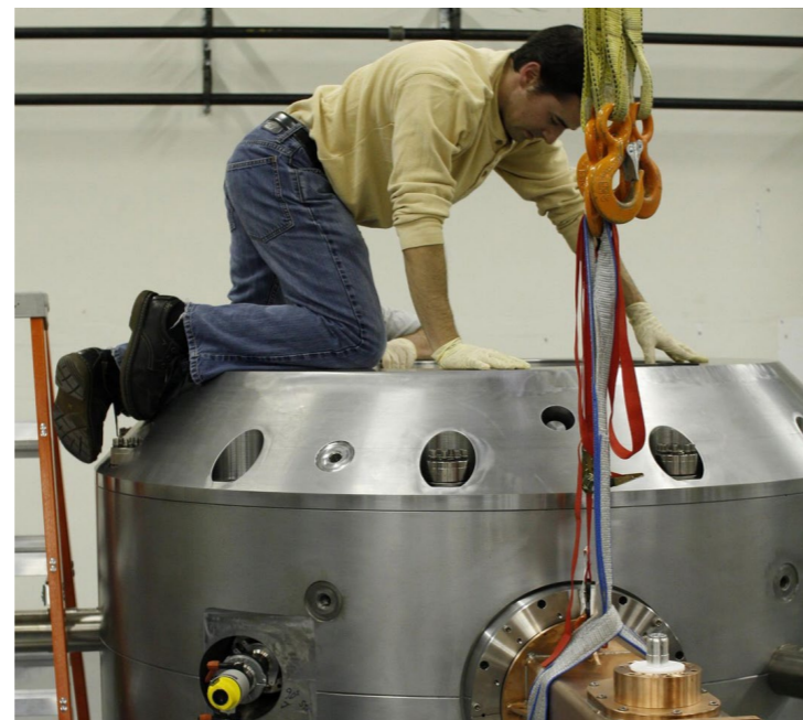
The single-gantry of ZON-PTC will consist of a Mevion device in which a 230 MeV proton cyclotron is mounted on a gantry.
