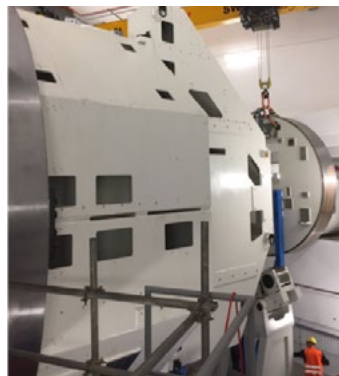
Gantry 2 being assembled
